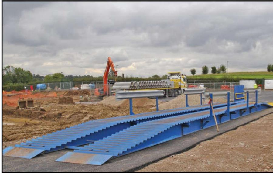
**Figure 4-1: Typical wheel wash using the dry ramp system**
